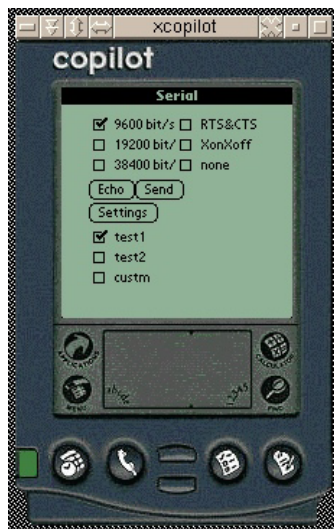
Figure 4-5 The test and configuration of the PalmPilots serial output with serial.c.
